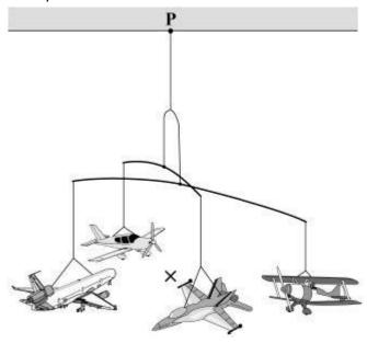
(ii) the centre of mass is (vertically) below the point of suspension / P
